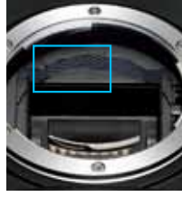
Vent for Airflow Control System
